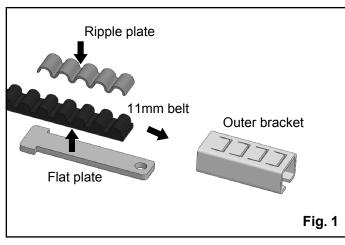
1. Attach the ripple plate and the flat plate on the belt as shown, and insert into the outer bracket.
