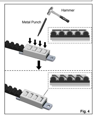
4. Set the bracket assembly on a hard wood or soft lead block.
