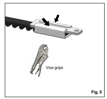
5. Use a pair of vice grips to crimp the spots as shown by the arrows on the back of the outer bracket. Deform the bracket for a firm assembly.
