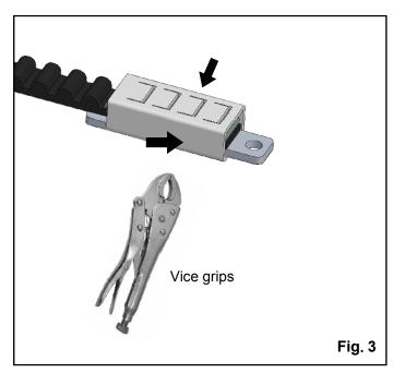
3. Use a pair of vice grips to firmly crimp the spots indicated by the arrows on the outer bracket.
