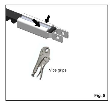
5. Use a pair of vice grips to crimp the spots as shown by the arrows on the back of the outer bracket. Deform the bracket for a firm assembly.
