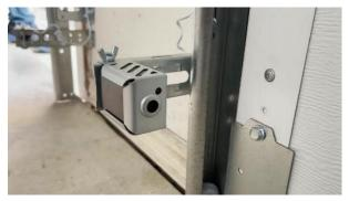
Another issue that can occur is when infrared radiation from the sun confuses the receiver. Direct sunshine on the RX can block the pulses from the TX. This is more likely to happen during sunrise or sunset when the sun is at the horizon.
