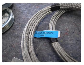
Another way to be effective is to carry common replacement components that do wear out and are typical serviceable items. Rollers, cables, and hinges would be at the top of this list. Other than that, you should carry sets of the regular common torsion springs for doors found in your local region. Because of the many door spring manufacturers scattered across the US, the
