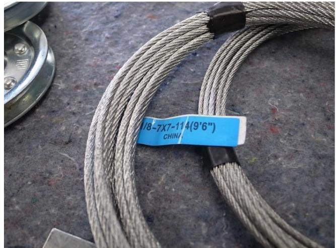
Another way to be effective is to carry common replacement components that do wear out and are typical serviceable items. Rollers, cables, and hinges would be at the top of this list. Other than that, you should carry sets of the regular common torsion springs for doors found in your local region. Because of the many door spring manufacturers scattered across the US, the
